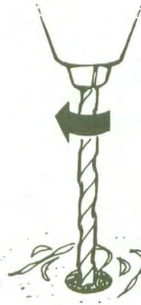
2. Drill hole in stud
