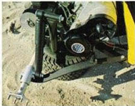
REAR SUSPENSION IS HEAVY DUTY LEAF SPRING AND AUTOMOTIVE SHOCKS
