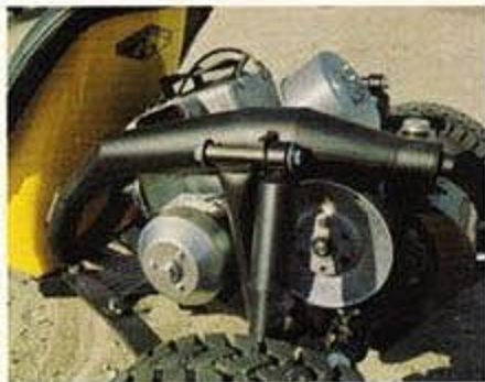
EXPANSION CHAMBER FOR GREATER POWER, BUILT IN MUFFLER AND U.S. FORESTRY APPROVED SPARK ARRESTOR
