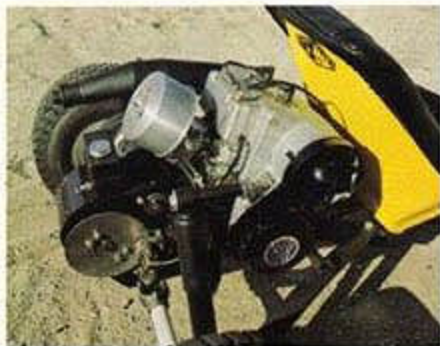
27 H.P. KOHLER SNOWMOBILE ENGINE WITH BUILT IN ALTERNATOR
