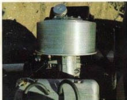
HEAVY DUTY AIR CLEANER FOR ENGINE PROTECTION AND WALBRÖ CARB. FOR SMOOTH PERFORMANCE
