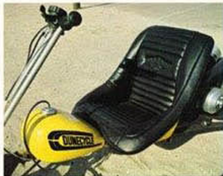
TWO GALLON REMOTE FUEL TANK, FUEL PUMP SUPPLIES ENGINE, HEAVILY CUSHIONED BUCKET SEAT FOR RIDING COMFORT.
