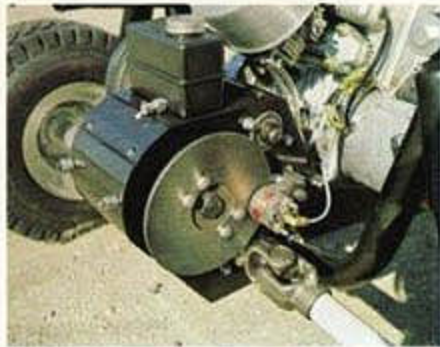
ENCLOSED DOUBLE JACKSHAFTS, CHAIN LUBRICATOR AND HYDRAULIC CALIPER DISC BRAKE
