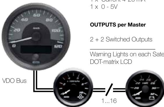
Up to 16 satellite gauges/master (Master can be Speedo, Tacho or Black Box)
