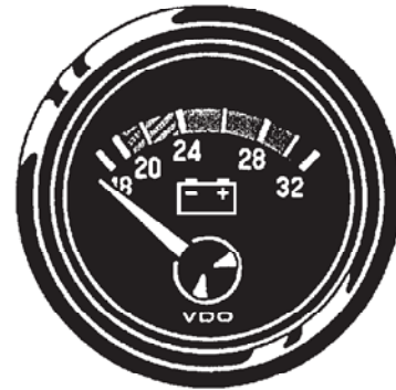
Example: voltmeter operating voltage 18 ... 32 V
