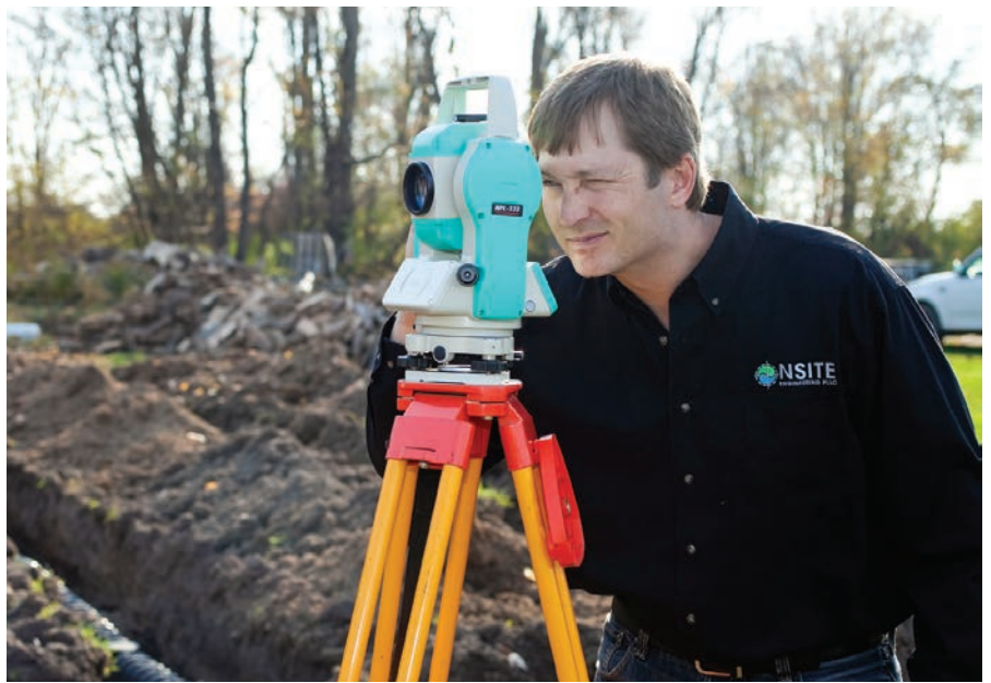
Murdock uses a Nikon NPL-332 Prismless Total Station for surveying to verify grades.
