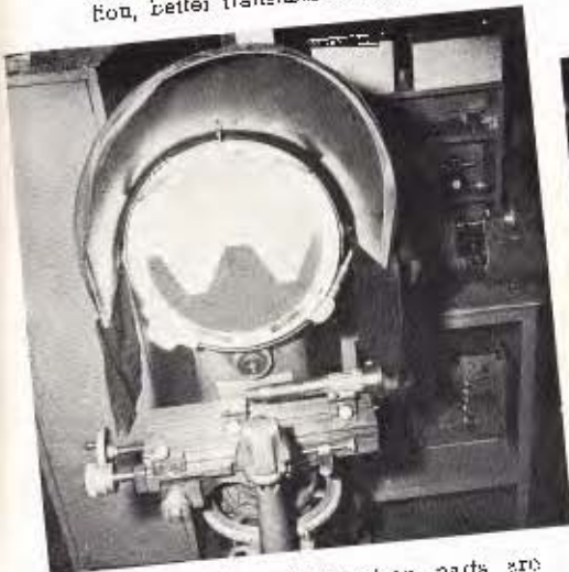
All machined and operating parts are checked by the highest standard gauges known. But to insure accuracy of fit of all parts, templates and thread contours are magnified E2\frac{1}{2} times.
