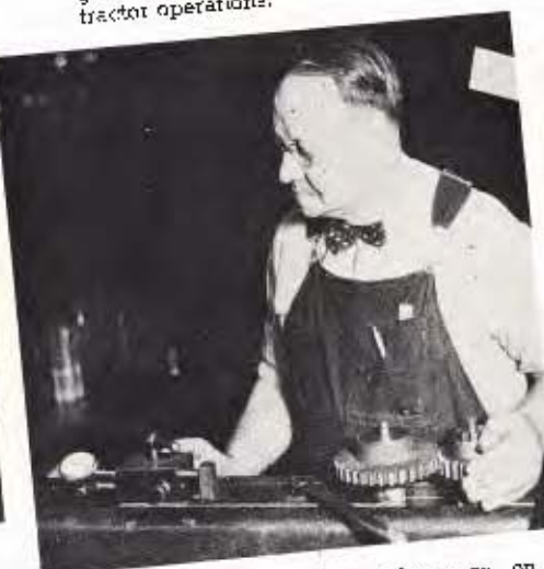
Correct "back lash," or clearance on making gears is constantly checked on the finest of precision equipment. The result is smooth, efficient power transmission.
