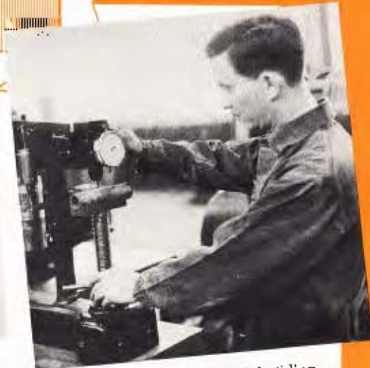
Nothing is left to chance in building Oliver "Cletracs." After heat treatment, track pins and bushings are Rockwell tested for proper hardness.
