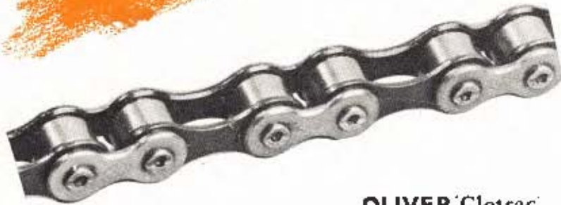
OLIVER "Cletrac" TRACKS ARE BUILT LIKE A ROLLER CHAIN
