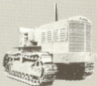
MODEL "F" SERIES Gas Diesel Drawbar H.P. Corrected to Sea Level... 51 56.5 Belt H.P. Corrected to Sea Level... 112.50 113.50 Approximate Weight... 27,000 28,120
