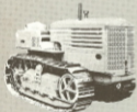
MODEL "B" SERIES Gas Diesel Drawbar H.P. Corrected to Sea Level... 25.0 22.2 Belt H.P. Corrected to Sea Level... 44 40 Approximate Weight... 3250 3060
