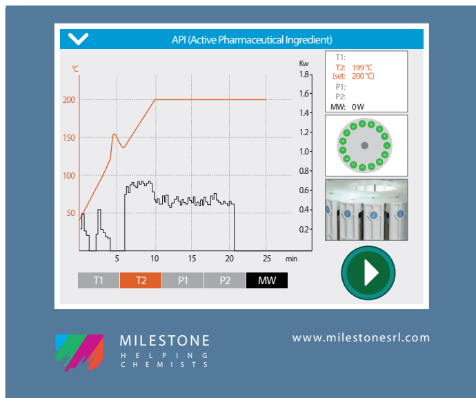
easyTEMP temperature control of an exothermic reaction during the digestion of an API with \text{HNO}_3 and \text{HCl} in the SK-15 rotor
