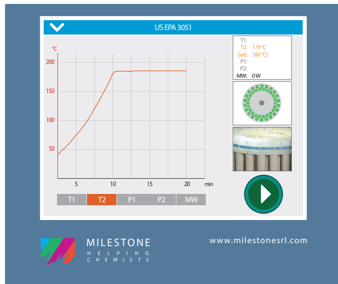
Temperature profile of a soil digestion in accordance with US EPA 3051 using the MAXI-44 rotor
