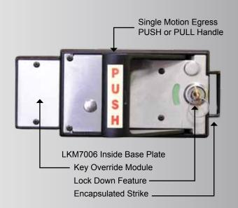
**Key Override Module** - Standard on the LKM7003 and 7006 Lock. This module "overrides" the access control device with the turn of a key, but not the combination lock. This feature is particularly important during the event of a power outage, failure or malfunction of an access control device, or an emergency that requires expedited entry.
