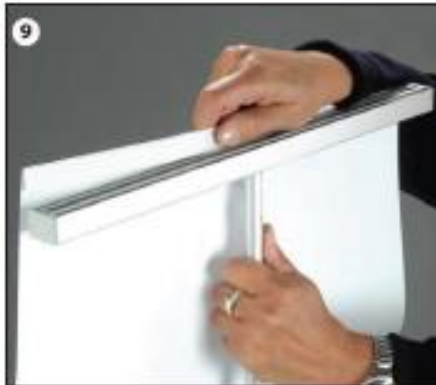
9 Push down on the top profile. The spring-loaded pole will adjust to the height of the graphic. Insert the edge of the graphic into the top of the structure (There are 3 slits in the top profile - place the graphics into the outer slits.) Repeat with second graphic.
