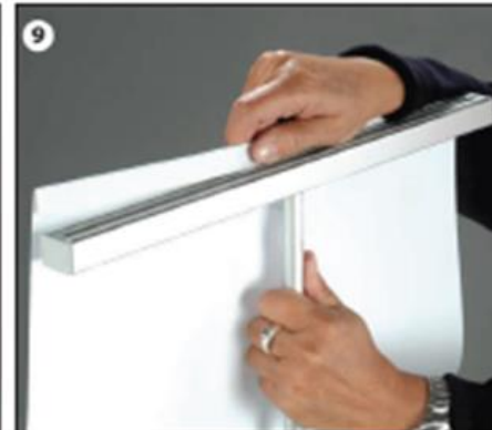
9 Push down on the top profile. The spring-loaded pole will adjust to the height of the graphic. Insert the edge of the graphic into the top of the structure (There are 3 slits in the top profile - place the graphics into the outer slits.) Repeat with second graphic.
