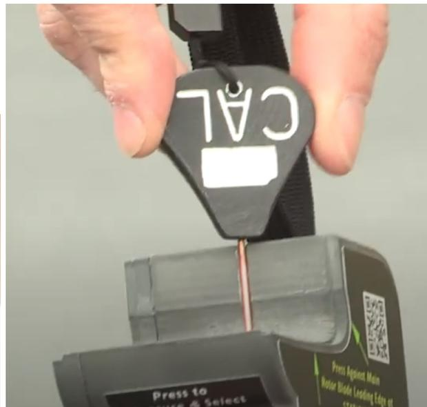
Press and release the function button once and wait for the word "good" to appear on the display panel.
