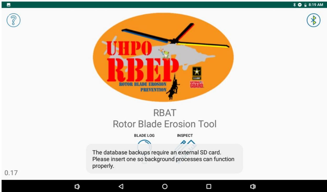
If this is the first time the SD card is being used, direct the system to store data in the RBAT directory on SD card. (See Transferring Data from the R-BAT Controller)
