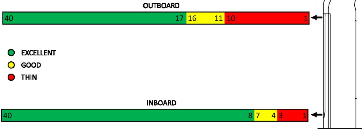
If Bluetooth communication cannot be established, the software allows for manual input of the R-BAT measurements and their LED ranking. In this case, use the RBAT tool to measure inboard and outboard locations of the nickel strip noting both measurement and rating color for each. Input this information manually on the measure page as shown below.
