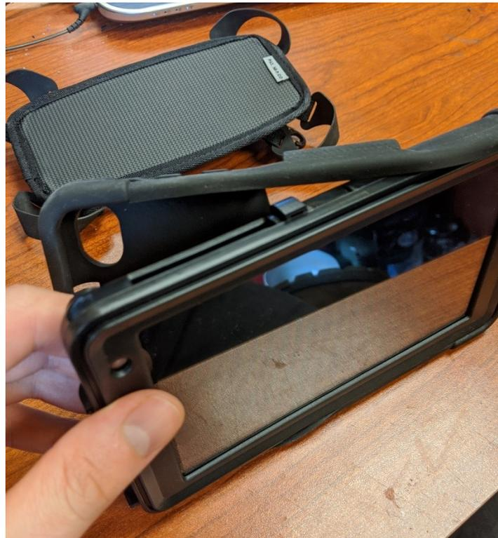
Then remove the controller's plastic outer casing by releasing the plastic case clips on each side of the controller. This can be done with a fingernail.
