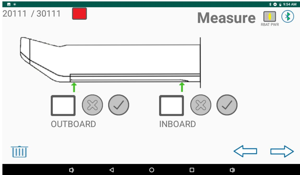
To take an “outboard” measurement of the nickel strip thickness:
