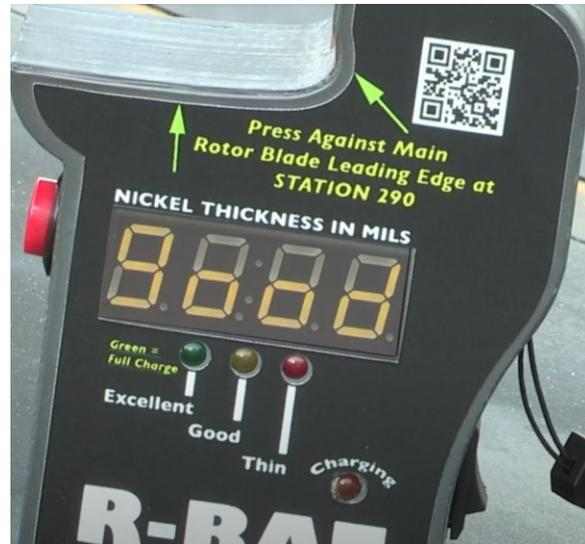
It may take the R-BAT up to 3 minutes to calibrate. If the unit fails to calibrate, the R-Bat will display redo. If this happens, remove the calibration key, press and hold down the function button for 3 seconds, and redo the calibration.
