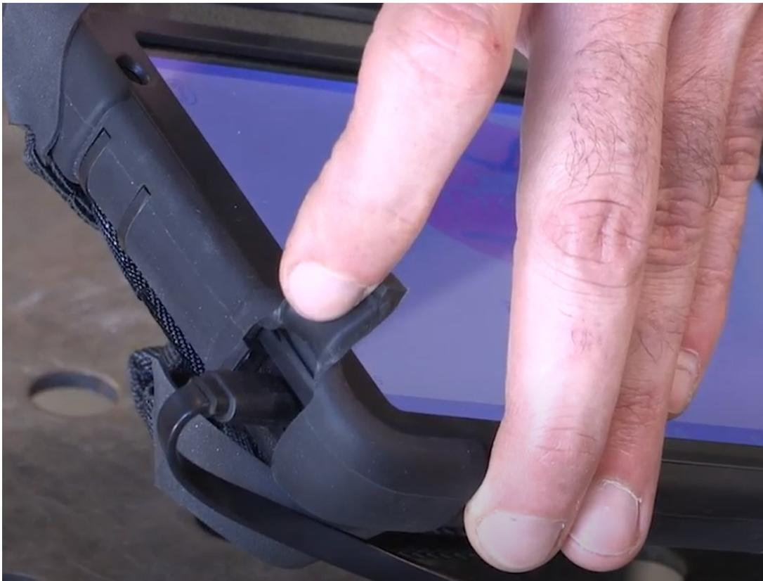
Once charged, ensure that a UPT-supplied SD card is installed in the controller and turn on the controller by pressing the power button. Next, select the R-BAT app on the touch pad. This launches the app and leads to the R-BAT homepage. If an SD card is not installed, the app will display the notification below, indicating that a SD card must be installed for the app to function properly.
