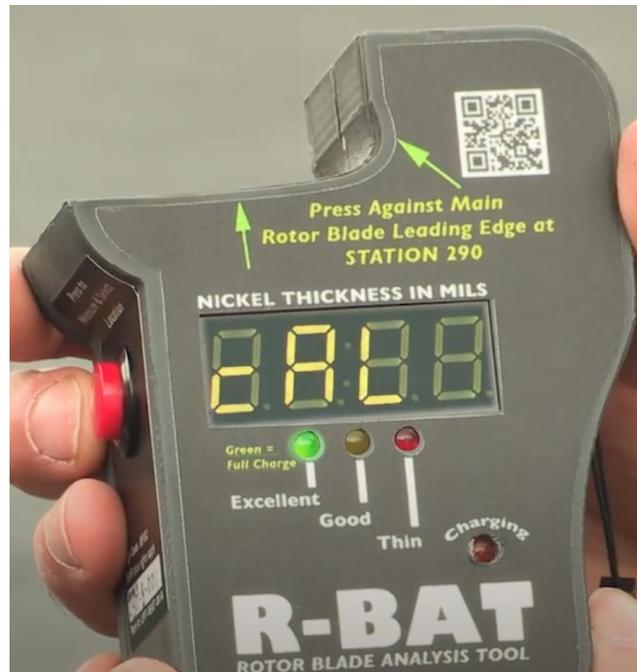
Remove the calibration key from the case and insert it into the calibration slot located on top of the R-BAT.
