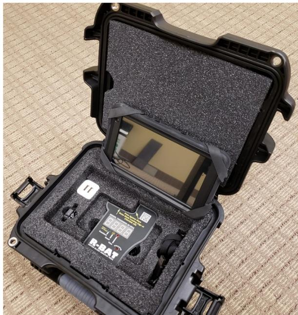
The R-BAT controller is equipped with a power button, charging port, Otterbox hand strap, and a tablet lanyard.
