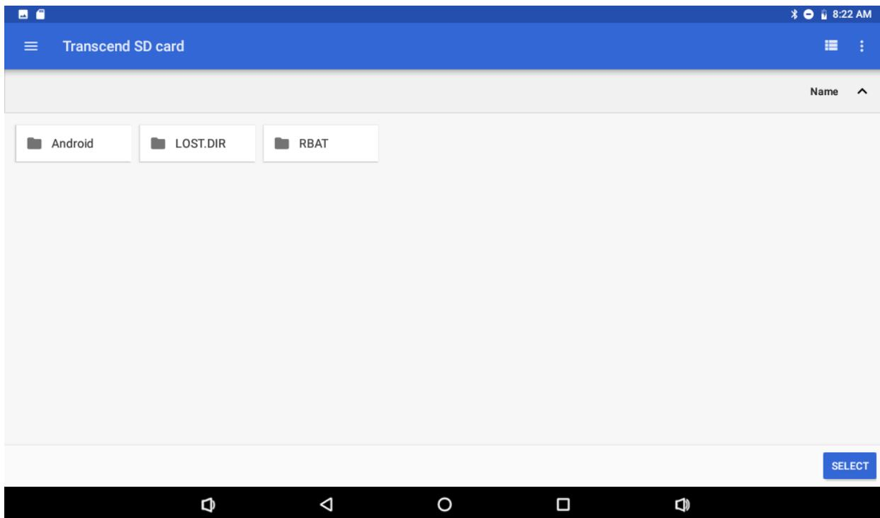
If a the user wants to use an SD card not supplied by UPT, the user must create a file named RBAT on the SD card to allow for file saving. Note that preloaded help options will not be available in this case.
