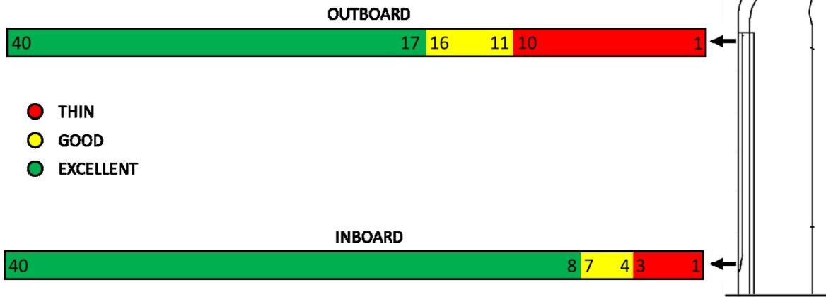
If “redo” is displayed on the panel, this indicates that the measurement lies outside the expected range of 1 to 40 mil and should be measured again. When “redo” is displayed the unit will also illuminate an LED indicating whether the measurement was below 1 (red) or greater than 40 mils (green).
