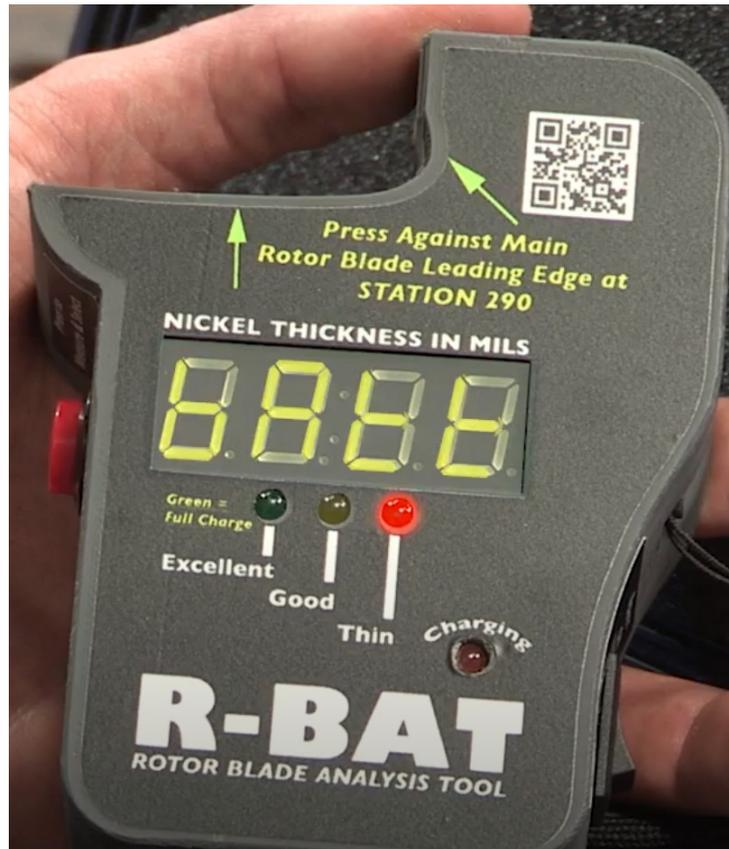
To recharge the R-BAT battery, press the power switch to the “off” position. Use the supplied USB charger by plugging the cable into the USB charge port located beside the power switch. Once the charger is plugged in, the LED labeled “charging” will illuminate. When the LED turns off, the charge is complete. Unplug the USB cable from the R-BAT charge port and switch the power “on” to determine the state of the charge. It can take a full 4 hours to charge the R-BAT.
