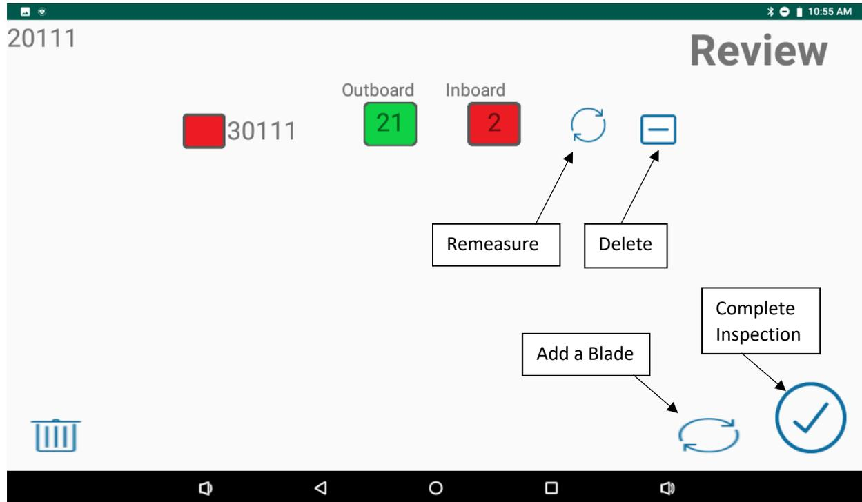
To remeasure inboard and outboard locations on a blade, press the circle located at the right of the blade. This will return to the pre-inspection page for that blade and allow replacement of the previous measurements of that blade.
