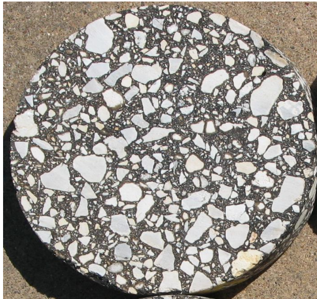
Warm Mix Asphalt
