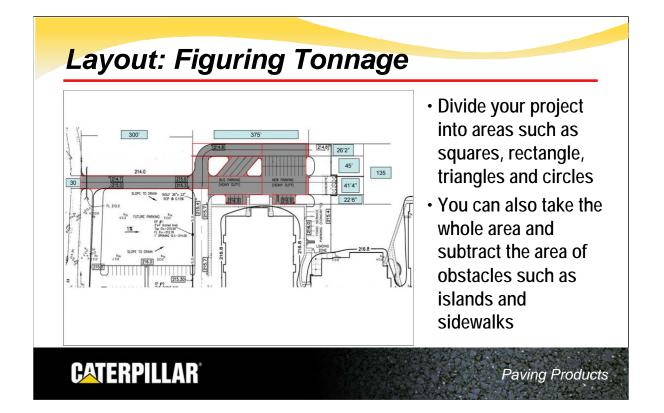
To calculate the paved surface area, divide the paved areas into geometric shapes such as squares, rectangles, triangles and circles. Another approach is to calculate the whole area and then subtract the area of the obstacles such as islands and sidewalks. Either method should produce the same square footage.
