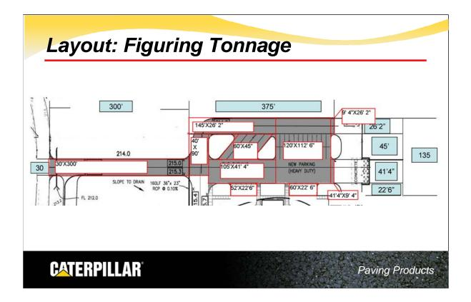
Using the dimensions of each area calculate the square footage. Round the measurements to whole numbers
