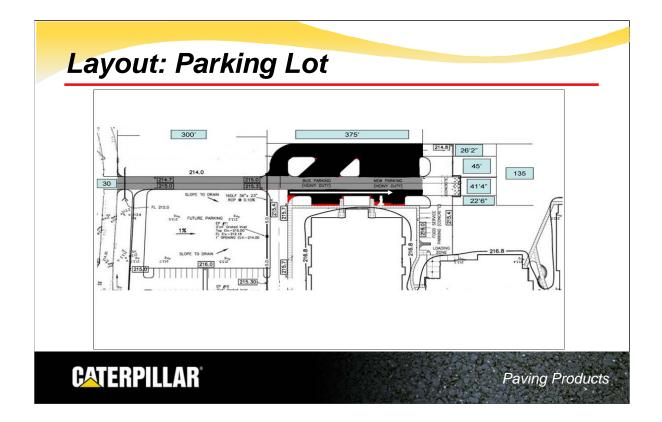
The crew was able to make one last long pull from left to right to finish the parking area. The starting pad was already there because the left end was the first paved in the lower lot. The crew is able to end the pull by taking the paver all the way up on the concrete apron.
