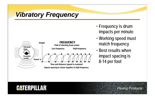
The other aspect of vibratory force is frequency. Frequency is defined as the number of times that the drum hits the mat and is rated in vibrations, or impacts, per minute.
