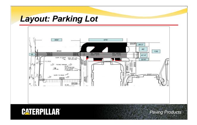
Moving across the lot the crew will continue to measure the remaining width and set up the screed to make pulls as evenly spaced as possible. The visual appearance is improved, plus the crew is trying to avoid, whenever possible, creating situations where they must overlap the previous mat (hot lap).
