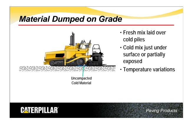
As the screed passes over these materials, fresh hot material is deposited over them. Any place the dropped material is thicker than the mat, it will be sheared off or will pick up the screed and not allow it to float properly. This will leave an area in the mat where the cold materials are just under the surface of the mat or are partially exposed.
