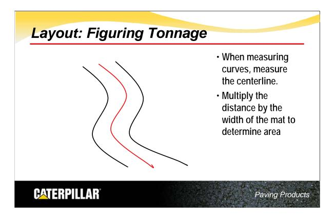
If there is a curved drive in the area to be calculated, measure the length of the curve at the centerline. Then, multiply that linear distance by the width of the mat to get the square surface area.
