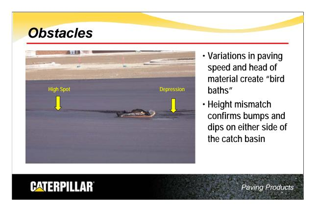
One of the worst flaws in a parking lot is a "bird bath" or depression. This view shows the high spot in front of the catch basin and the dip behind the catch basin. These mat defects are common and are caused by changes in paving speed and head of material. Part of the problem is also due to the hand work done prior to paving. There is one more lift to try to get it right, but the low spots will still compact down to low spots in front of the catch basin.
