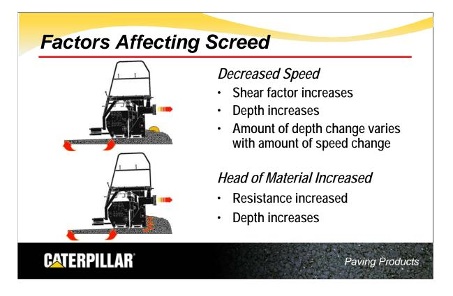
When the paving is decreased, the shear factor acting on the front of the screed increases. Less mix can pass under the nose of the screed and the screed rides up. The distance that the screed climbs depends on how drastically the speed is reduced.
