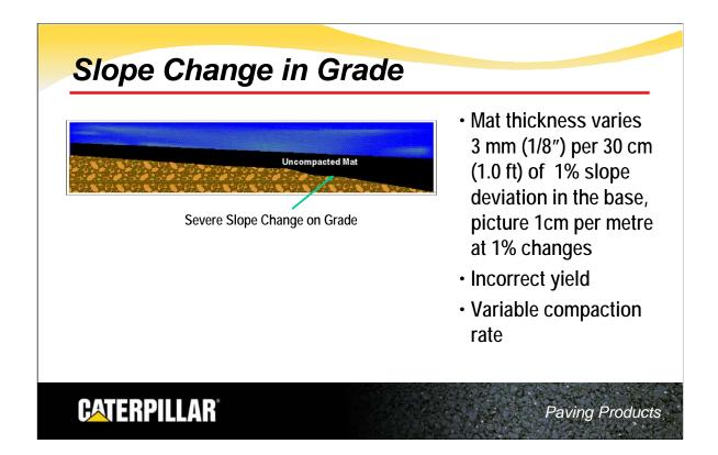
The slope of the existing grade may create a problem if it varies significantly from the mat placed over it. For example, if the slope of the grade is running at 4% and a mat with 2% slope is placed over it, the mat thickness will vary correspondingly. Or, if the slope of the grade changes significantly at some point, the mat thickness will change at that point also. The mat will compact at a different rate and it is likely the specifications for density and yield will not be met.
