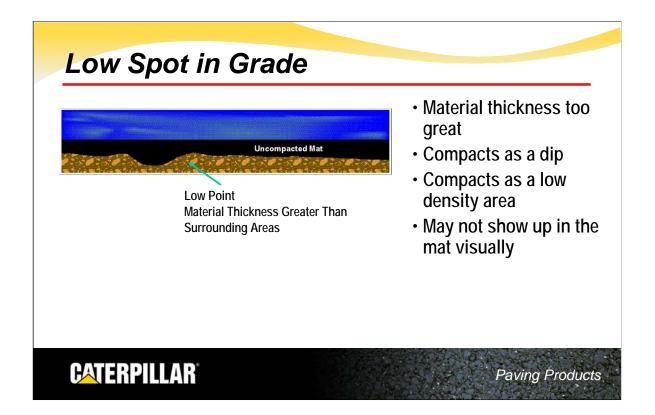
When a mat is placed over a low point in the existing grade, the material thickness is greater than the surrounding areas. When compacted, these areas will compact at a higher rate and a dip will be produced. If the low spot is smaller in diameter than the width of the roller, the roller will bridge over the low spot and a low-density area will result.
