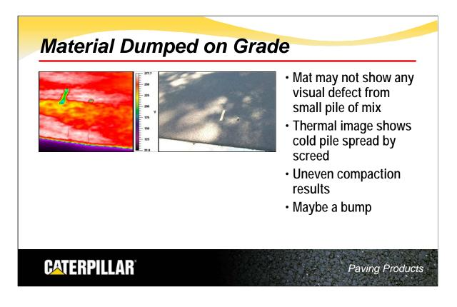
Visual inspection of the mat (photo on right) may not show any apparent defect since the material dumped on the grade has been "buried". But, a thermal image of the same area (left photo) reveals a cold streak where the dumped material has been leveled and spread by the screed. The cold area will not compact the same as the rest of the mat. A bump can be produced.
