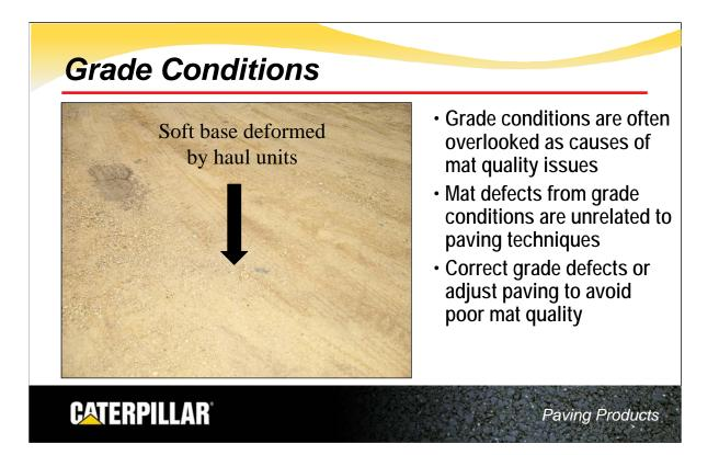
No structure is stronger then the foundation on which it is built. The same is true with asphalt paving. To produce a quality mat, there must be a quality foundation or "base" to build on. Grade conditions will be reflected in the mat. Sometimes these defects show up immediately and at other times they take longer. Let's discuss how different grade defects can result in poor quality mats and premature failures.
