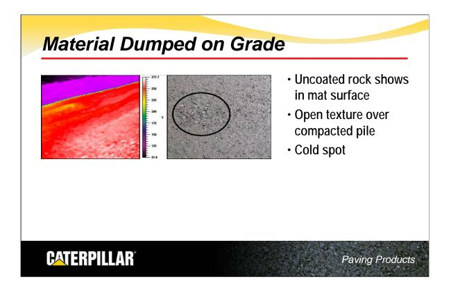
Because the mat is so thin over the pile of pre-compacted asphalt, the force of the compactor can fracture aggregates. The area in the mat that has been circled contains fractured aggregate which show as uncoated rock surfaces.
