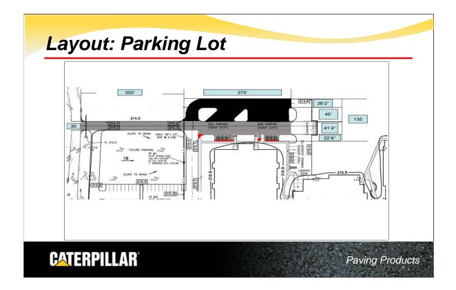
Now the crew moves to the lower portion of the parking lot where more hand work is needed. At the left end, the tapered area will be filled by hand. The tapers in the center and the area between the sidewalks also get filled in by hand. Both lower parking areas will need pads built for starting reference as no suitable reference exists.
