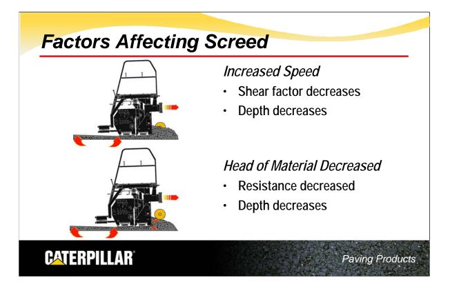
As paving speed increases, the shear factor decreases. More mix gets pushed in front of the screed and less mix passes under the nose of the screed. Consequently, the depth of the mat decreases until all the forces acting on the screed stabilize.
