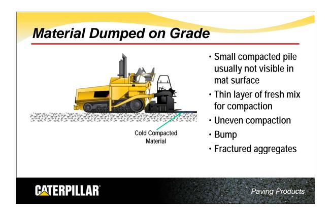
As the screed passes over the compacted pile, hot material is deposited over it. Normally, the small pile is undetected in the mat. But when the roller passes over the pile, the thinner layer of fresh material can not be compacted at the same rate. A bump may be created and aggregates may be fractured, too.
