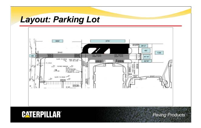
The last pull completes the area. The screed width had ample extension left to correct the final pull width. A small amount of hand work is required at the ends of the curved island.
