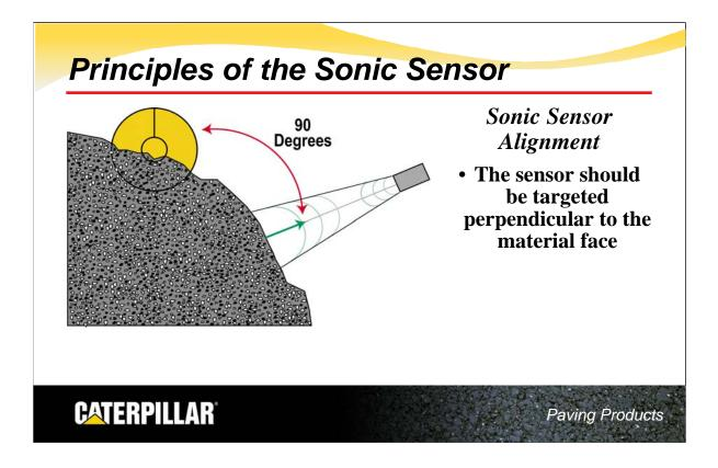
The sonic sensor must be installed so the sensor is perpendicular to the target. The sensor emits 40 sound pulses per second and expects to receive 40 returning echoes in order to make accurate calculations. When the sensor is aimed incorrectly, some of the sound pulse echoes do not go back to the sensor. Lacking full information from the sensor, the feeder system acts erratically.
