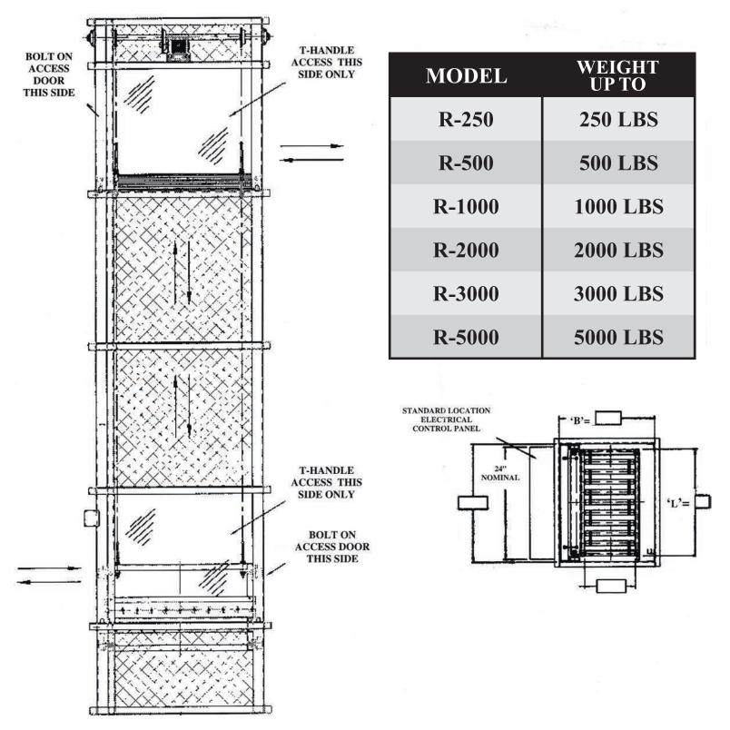
Material Lift, Dumb Waiter, Mezzanine Lift
