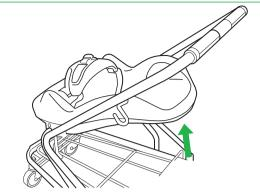
③ Push the top of the seat upward from the rear to check that it stops in each reclining position (medium and upper positions).
