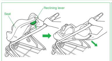
① Raise the reclining lever to check that the lock is released, and, with the lever in the raised position, lower the seat to check that it reclines (3 positions).
