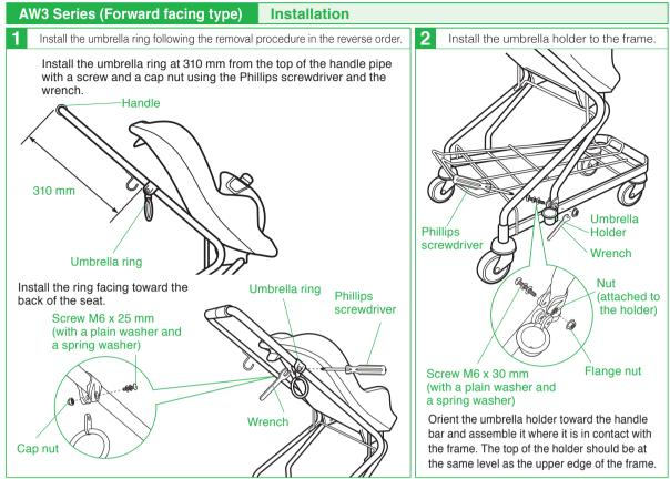
Note: The screw used for the umbrella ring and the one used for the umbrella holder do not have the same length. Pay attention to use the correct screw for each part.
