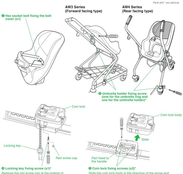
Remove the red screw cap at the bottom of the coin lock to reach to the locking key fixing screw.
