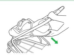
④ If the seat does not stop at the three reclining positions or it moves to a position almost horizontal, or if it rotates to the bottom side, it means that the seat is defective. In such a case, stop immediately using the Product and contact the CombiWith Service Center.
