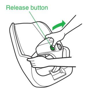
③ Press the release button and pull the guard toward you while holding the seat with one hand to check that the guard opens.
