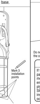
Temporarily remove the base, and install 3 anchor bolts in the marked areas.
