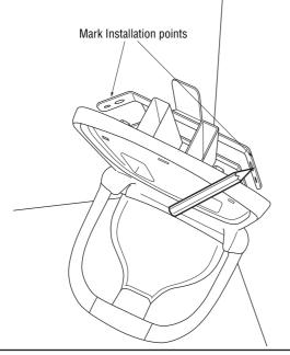
Fix the corner fixtures to the wall at four mounting points.
