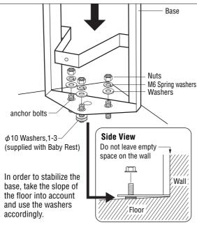
Once the corner fixture is mounted onto the wall, connect the base.
