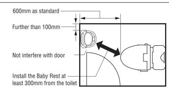
• Install on a wall at least 600mm away from the toilet, or insure 300mm of space between the Baby Rest Fit FL and toilet.
