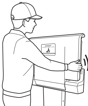
② Close the table and shake to check the rattling.
