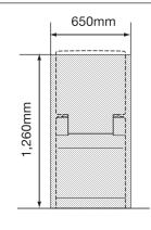
When using tapping screws to mount the product on a partition wall, insert a reinforced wood of 30mm or more without any space at the tapping screw fixing position.
