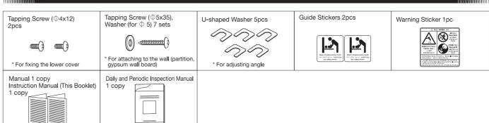
• Anchor bolts are not included. Prepare separately. Use 3pcs of M10 for floor and 6pcs of M6 to M10 for concrete wall and ALC. (Refer ② of "List of Mounting Screws for the Wall" above)
