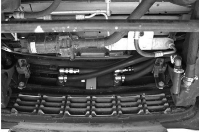
Photo showing heat exchanger removed with all KC lines connected.
