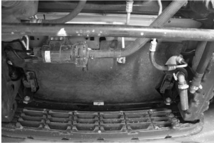
Rubber shield installed.
