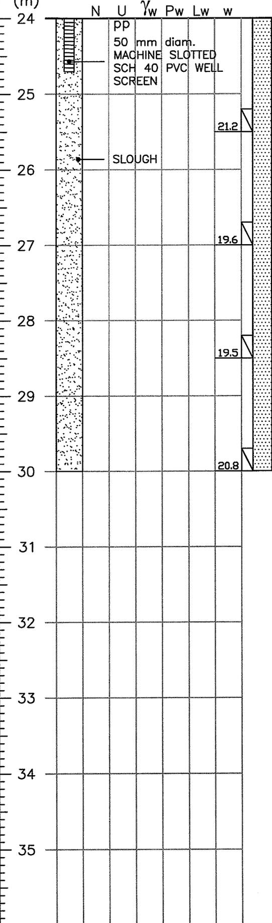
**SAND**, silty, some gravel, trace clay, very dense, well graded, fine to coarse grained, wet, grey, seepage, sloughing.
