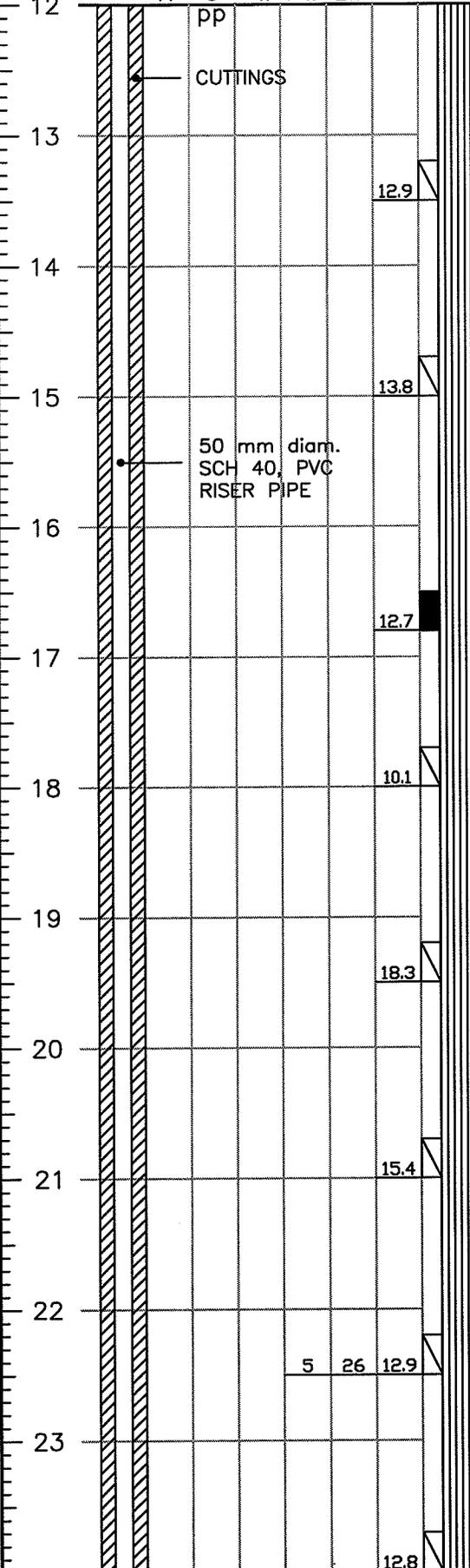
**SILT**, some clay, some sand, hard, medium plastic, moist, brown, oxide stained.
