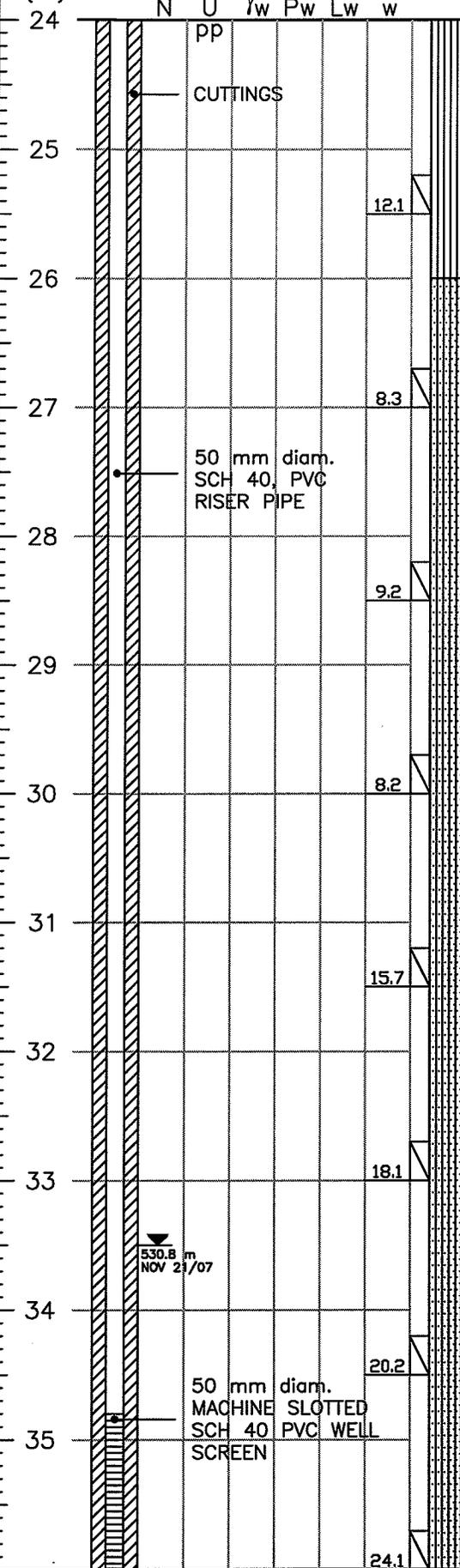
**SILT**, some clay, some sand, hard, low plastic, moist, brown, oxide stained.
