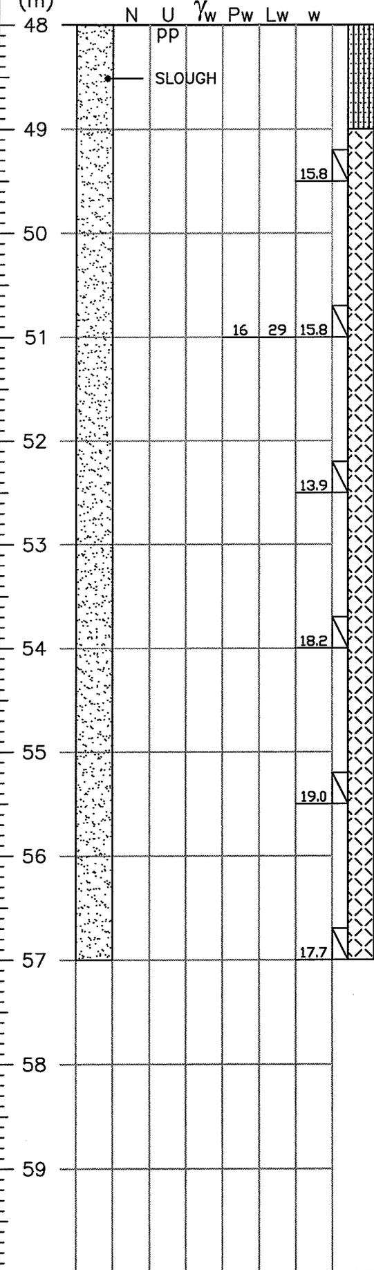
**SAND AND SILT**, dense, poorly graded, fine grained, wet, grey, seepage, sloughing.
