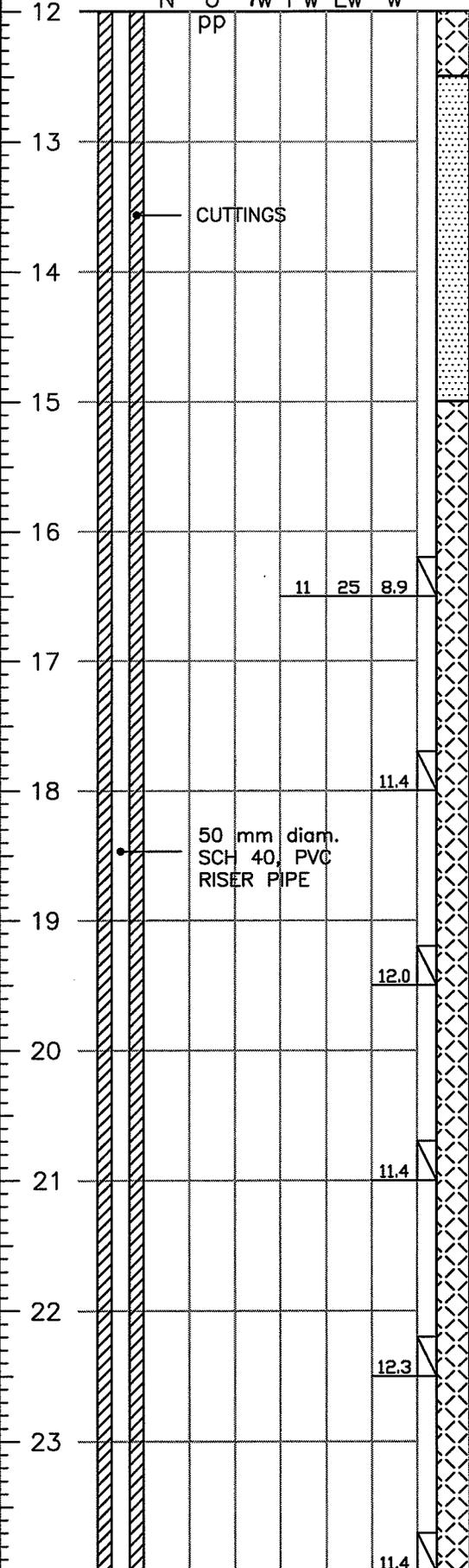
**GLACIAL TILL**, clay, silty, sandy, trace gravel, very stiff to hard, low plastic, moist, brown, oxide stained. **SAND**, some gravel, dense, well graded, fine to coarse grained, damp, brown.
