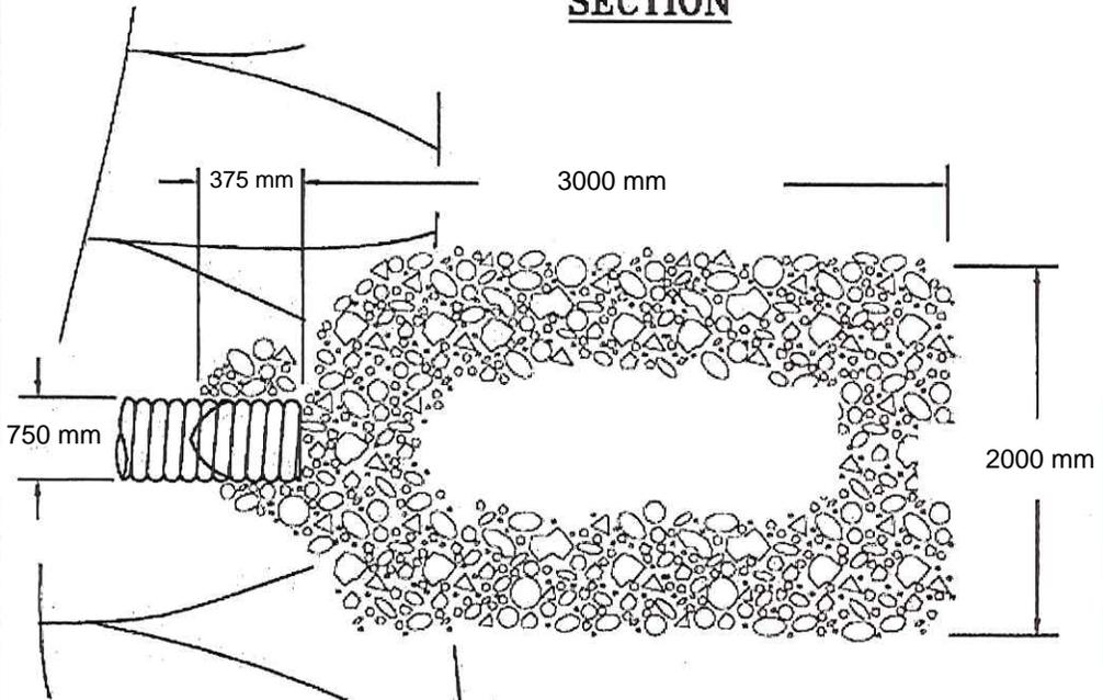
***FILTER AND ROCK LAYER MUST BE CONTINUOUS AND MAINTAIN INTIMATE CONTACT WITH THE BASE SOIL OR FILTER LAYER. GRANULAR FILTER DETERMINED BY QUALIFIED PROFESSIONAL. MIN. THICKNESS 150 MM. WOVEN OR NON-WOVEN GEOTEXTILE MUST MEET SPECIFIED MATERIAL PROPERTIES.***
