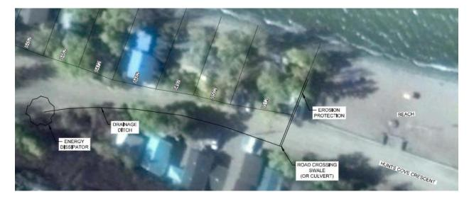
Figure 5.3: Drainage Ditch Option, crossing at beach
