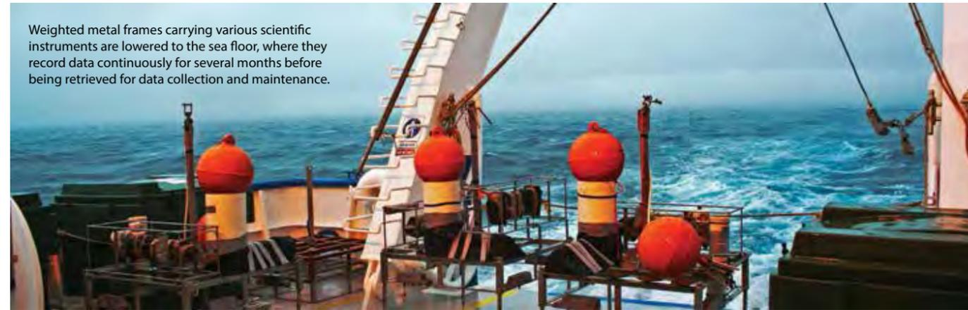
Weighted metal frames carrying various scientific instruments are lowered to the sea floor, where they record data continuously for several months before being retrieved for data collection and maintenance.
