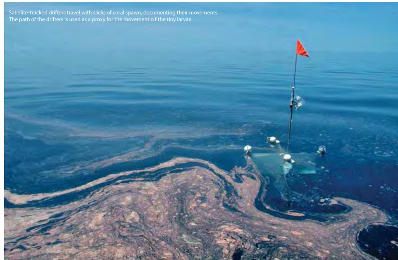
Satellite-tracked drifters travel with slicks of coral spawn, documenting their movements. The path of the drifters is used as a proxy for the movement of the tiny larvae.
