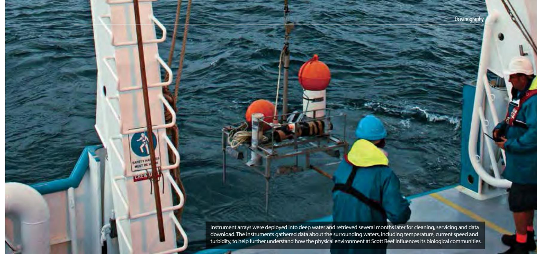
Instrument arrays were deployed into deep water and retrieved several months later for cleaning, servicing and data download. The instruments gathered data about the surrounding waters, including temperature, current speed and turbidity, to help further understand how the physical environment at Scott Reef influences its biological communities.
