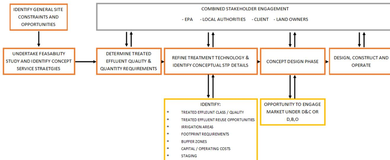
Figure 9 Sewage Treatment Plant Selection and Design Process Flow Chart
