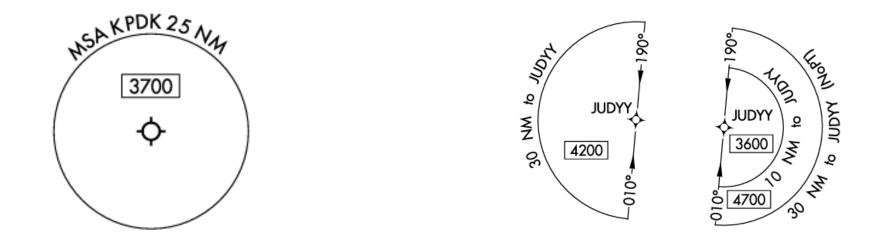
The MSA (Minimum Safe Altitude) circle appears in the plan view except in approaches for which the navaid is unavailable.
