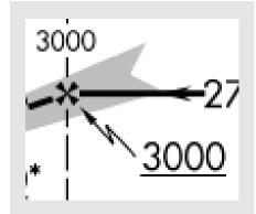
Lighting bolt = precision FAF determined by altitude Which is determined by altimeter setting
