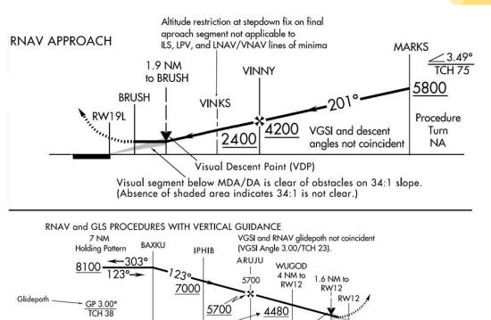
Altitude restriction at stepdown fix on final Visual Descent Point (VDP) approach segment not applicable to ILS, LPV, Visual segment below MDA/DA is clear of obstacles on 34:1 slope. and LNAV/VNAV lines of minima (Absence of shaded area indicates 34:1 is not clear.)
