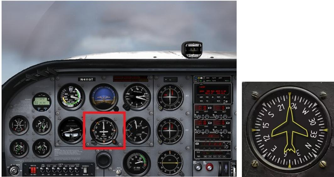
The heading indicator is a flight instrument used in an aircraft to inform the pilot of the aircraft's heading. It is sometimes referred to by its older names, the directional gyro or DG, and also direction indicator or DI.
