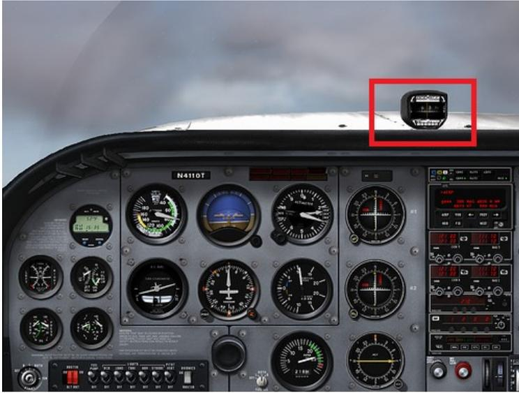
You will find a magnetic compass on top of the dashboard of the aircraft or mounted at the top of the front window. You would think that the more expensive instruments in the dash would be more accurate but usually you adjust other instruments based on this.
