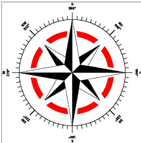
A compass divided into 360 degrees is the most common unit of measurement. Each degree is divided into 60 minutes, each minute into 60 seconds. A handheld compass is not able to measure down to a minute, let alone a second, but those units are used for precise locations using latitude and longitude.
