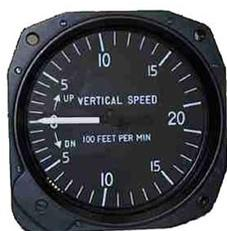
The Rate of Climb and Rate of Descent are indicated on the Vertical Speed Indicator (VSI). This is measured in Feet Per Minute, and displayed in Hundreds of FPM.
