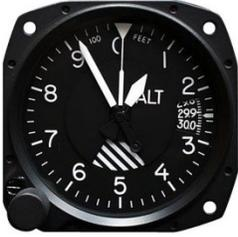
The altimeter simply indicates the height in feet above sea level. Altitude can be determined based on the measurement of atmospheric pressure. The greater the altitude, the lower the pressure. When a barometer is supplied with a nonlinear calibration so as to indicate altitude, the instrument is called a pressure altimeter or barometric altimeter.
