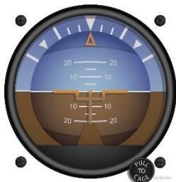
An attitude indicator (AI), also known as gyro horizon or artificial horizon is an instrument used in an aircraft to inform the pilot of the orientation of the aircraft relative to Earth's horizon. It indicates pitch (fore and aft tilt) and bank (side to side tilt) and is a primary instrument for flight in instrument meteorological conditions.
