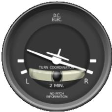
In aviation, the turn and slip indicator (T/S, a.k.a. turn and bank indicator) and the turn coordinator (TC) variant are essentially two aircraft flight instruments in one device. One indicates the rate of turn, or the rate of change in the aircraft's heading, the other part indicates whether the aircraft is in coordinated flight, showing the slip or skid of the turn.
