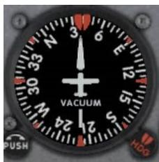
The magnetic compass is the primary direction indicator in an aircraft, but it is prone to a number of errors due to acceleration and turbulence. The can also be hard to read especially when the sun is bright or it is night. We use a direction indicator based on a gyro. They are stable, usually accurate, and easy to read. The can be synced to a magnetic compass in some cases.
