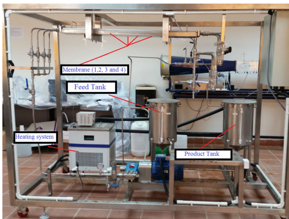
Fig. 4 The membrane filtration test unit; Model: TR 14
