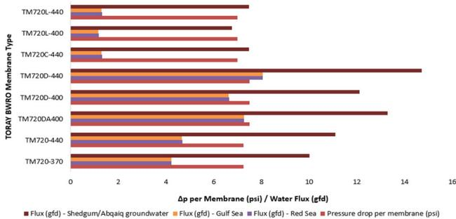
Fig. 2. Observed water flux for various water sources at different applied pressures using Toray BWRO membranes.
