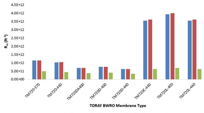
Fig. 3. Observed membrane resistance of various water sources in Toray BWRO membranes.
