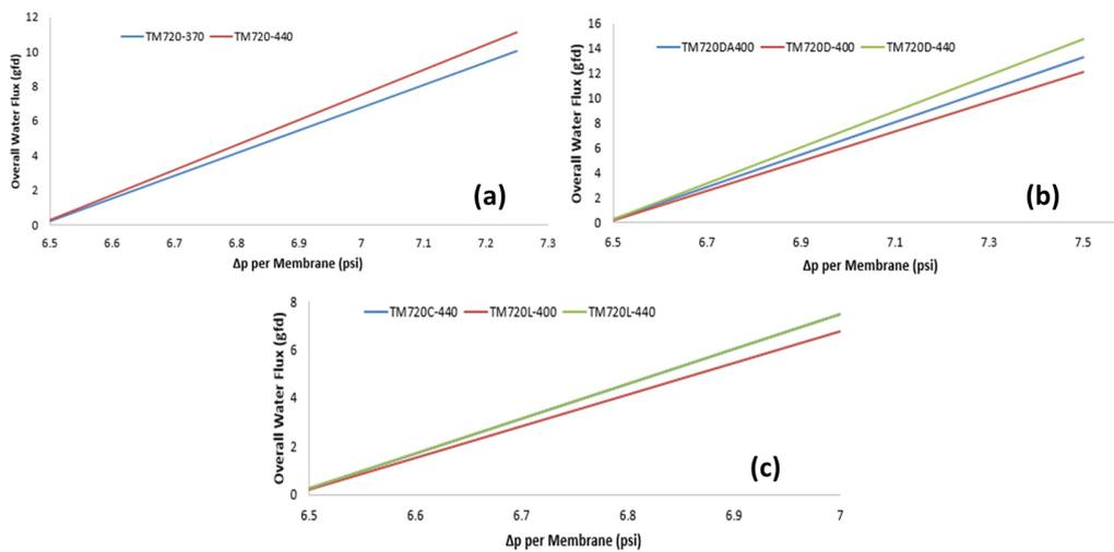
Fig. 1. Effect of different applied pressures on the groundwater flux for (a) Toray standard BWRO membranes, (b) Toray high-pressure BWRO membranes, and (c) Toray low-pressure BWRO membranes.
