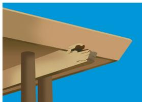
7. If the rot cavity is dry from step 5, measure the **RotFix**® (2 Parts A to 1 Part B) and mix thoroughly. Apply 1 or more coats of **RotFix** to the cavity and lightly brush over the surface of the **Bor8rods**® holes being careful not to get any down in the hole. **RotFix** will harden the wood and create a chemical and mechanical bond between the **SculpWood**® and the original wood.
