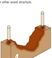
Bor8rods inserted into drilled holes.
