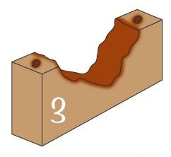
Board Defense® solution applied to rot cavity and into holes for Bor8rods.
