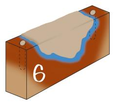
Overfill cavity with SculpWood™ putty and/or paste. Seal Bor8rod holes.
