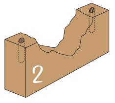
Rotten wood removed. Holes drilled for Bor8rods® .
