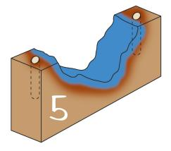
RotFix™ applied to surface of cavity. Apply a small amount to the surface of Bor8rod holes.
