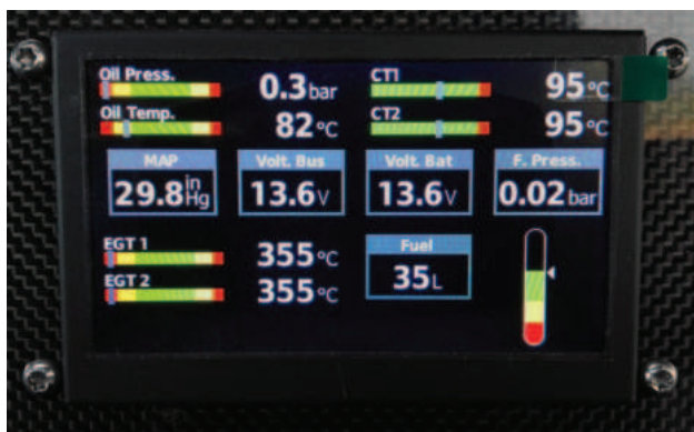
ALPHA Trainer Engine Management System display (example of data presentation via Kanardia DIGI display)
