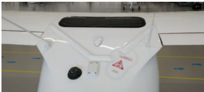
BPRS installation: hatch and belt positioning
