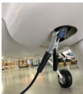
Ground wire connected to exhaust.
