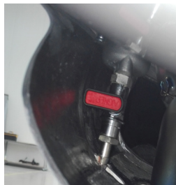
Fuel/water drain outlet
