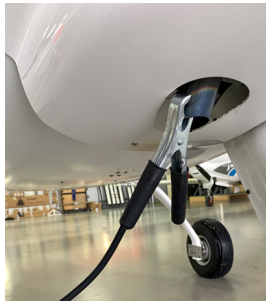
Ground wire connected to exhaust.
