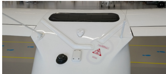
BPRS installation: hatch and belt positioning
