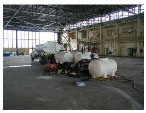
Each well was estimated to have a radius of influence of approximately 10 feet each. Over the course of this project, a total of 75,000 pounds of sodium persulfate and 15,000 pounds of ferrous sulfate were mixed into solution and injected into the groundwater. The injections were completed over a period of 41 days in the field.
