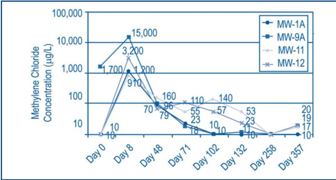
Figure 2. Although three of the four ISCO monitoring wells showed slight rebound at different times (likely due to back diffusion from clay), methylene chloride concentrations in all four wells remained steadily below 50 mg/L one year after the injections.
