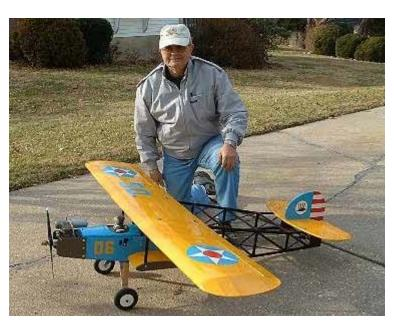
fuselage, and a parasol wing. It looks like something out of the deep past. It weighs in at 10 pounds and is powered with a Super Tigre 90. It has a 72 inch flat bottomed wing and should fly like a trainer...we'll see.
