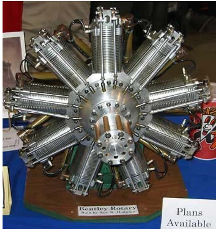
**9 Cylinder Rotary Engine**
