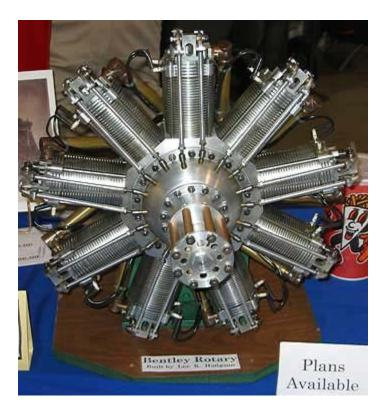
9 Cylinder Rotary Engine
