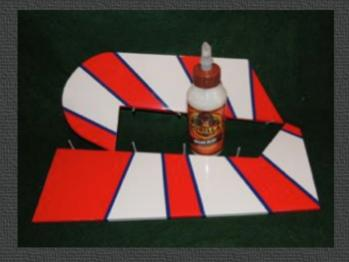
I started to apply CA to all of the joints. Besides having limited space for my hands, I found that I was chasing the fuse all around the work bench because the bottom of the fuse is rounded and it won't hold still. So I installed the main gear,
