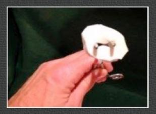
Feed the servo wire thru the slit and then glue the wire keeper to the inside of the hole.
