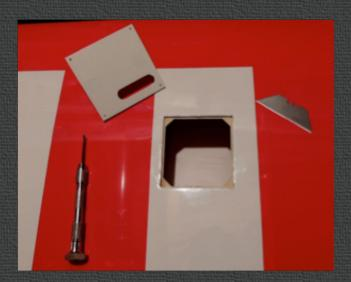
The hatch covers have a built in servo mount but it didn't allow enough room for my servos. So I removed the blocks and repositioned them with epoxy.
