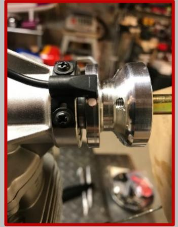
This only works for engines with slotted hall sensors like DLE, Zenoah, and RCG engines. It will not work on DA engines as they have preprogrammed timing maps and they also will not put out a spark until the engine sees 150 rpm, (basically the speed it is while flipping a prop manually). Do not be overly concerned if you can't get it perfect, the slotted Hall sensor does not have enough variation in the adjustment to harm the engine. Only about 3-4 degrees.
