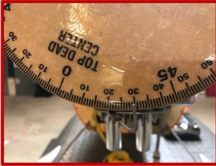
several times to find the exact point at which it fires. A properly set timing should be around 28-30 degrees before TDC. If it fires at 35 degrees, or higher, it is too far advanced. Loosen the screws holding the Hall Sensor, (nothing more than a magnetic on-off switch) which has slots for adjustment, and move the Hall Sensor in the same direction as normal rotation to retard the timing. If it is firing late or retarded, it should be moved in the opposite rotation to the advance timing.
