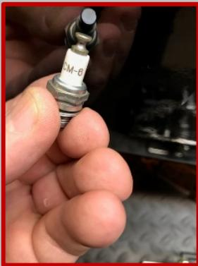
Never rotate a gas engine with the ignition system on and no plug in the plug holder. This will cause the capacitor inside the ignition box to discharge and burn out. The metal casing around the plug wire is the ground for the system.
