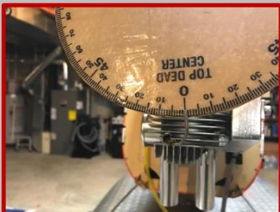
Once TDC is established. Put the spark plug into the plug cap and properly re-seat it. With the ignition turned on, rotate the crankshaft around about 75 degrees from TDC and then rotate the shaft in a normal rotation direction up to the 28-30 degree mark and you should hear an audible click from the spark plug or see the spark plug fire. Sometimes it is very hard to see the spark fire unless it's dark. Do this
