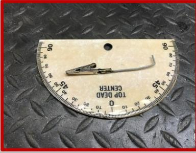
The first thing to do is remove the spark plug and find TDC of the piston. Remember, TDC is the furthest a piston will travel upward in the cylinder.
