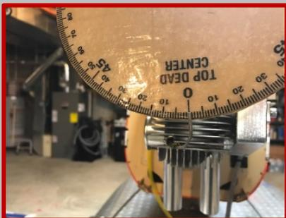
Once TDC is established. Put the spark plug into the plug cap and properly re-seat it. With the ignition turned on, rotate the crankshaft around about 75 degrees from TDC and then rotate the shaft in a normal rotation direction up to the 28-30 degree mark and you should hear an audible click from the spark plug or see the spark plug fire. Sometimes it is very hard to see the spark fire unless it's dark. Do this
