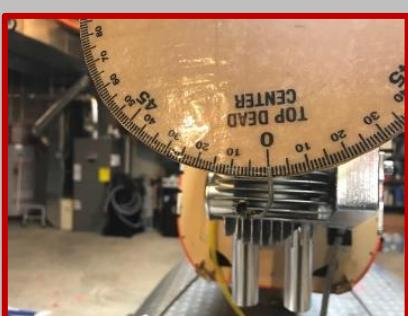
**Once TDC is established. Put the spark plug into the plug cap and properly re-seat it. With the ignition turned on, rotate the crankshaft around about 75 degrees from TDC and then rotate the shaft in a normal rotation direction up to the 28-30 degree mark and you should hear an audible click from the spark plug or see the spark plug fire.**
