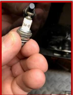
**Some of the other pictures are of proper plug to cap seating and other components of a typical capacitive discharge ignition system. As much as I like DLE engines, the spark plugs that come with them are guaranteed to fail prematurely. Replace them with an NGK CM-6 or Nippon Denso plugs. Always make sure your wiring is tied down to something, i.e. Zip-Ties or sticky back hold downs.**
