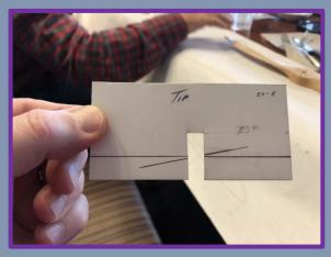
Leo said he researched the design and dimensions required to make the propellers that can withstand the stress and provide the correct performance for an RC model gas engine. He made various prop dimensional and airfoil templates and divided the prop into quarter sections that allow for easy airfoil shaping with sanders.
