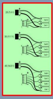
charger can read the voltage for each individual cell in the battery pack and adjust their individual voltages as needed, thus <u>balancing the battery pack cells</u>.
