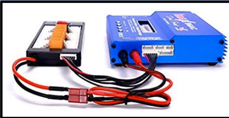
***Example: Single Port battery charger with a 6 Port XT-60 Parallel Balance Port Charging board connected. Batteries will connect to the Parallel Charging Board.***
