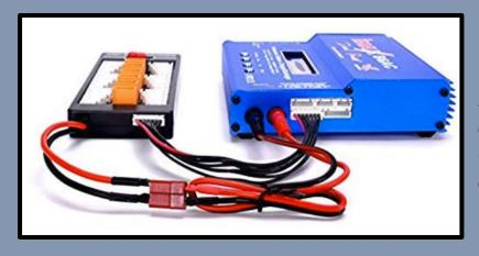
Example: Single Port battery charger with a 6 Port XT-60 Parallel Balance Port Charging board connected. Batteries will connect to the Parallel Charging Board.
