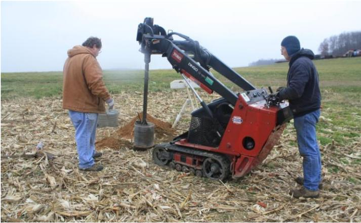
*The auger at work drilling a hole.*
