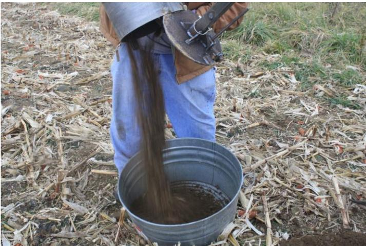
*Emptying the soil from the auger bucket.*
